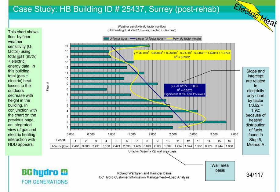
This chart shows floor by floor weather sensitivity (U-factor) equal to the overall enclosure value. For each floor. common area das consumption depends on variables such as air leakage, operable windows. and ventilation. The electrical consumption is an index of how much additional heat was needed to match aggregated suite thermostat set points given that the building is constantly losing heat to the environment according to the enclosure's steadystate thermal transmittance (Ufactor).
