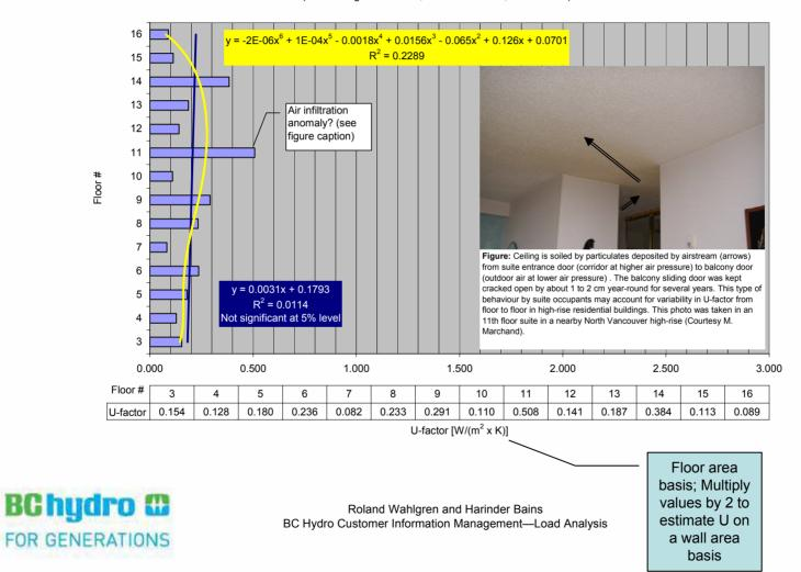
Weather sensitivity (U-factor) by floor (HB Building ID # 212087, North Vancouver, Electric heat)
